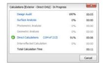
When changes have been made to the lighting *model* that require a re-calculation, Visual will indicate that **Calculation Zone** values may no longer be valid by bracketing point values.
